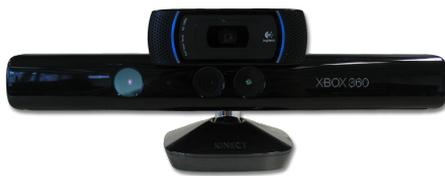
Figure 3: Sensor unit with a Kinect and a Logitech C910 web-cam.
