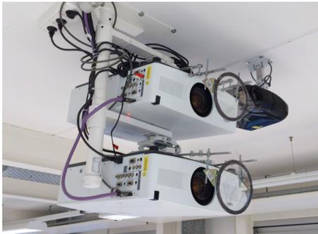
Figure 1: The two projectors for 3d projection with the polarizing filters.
