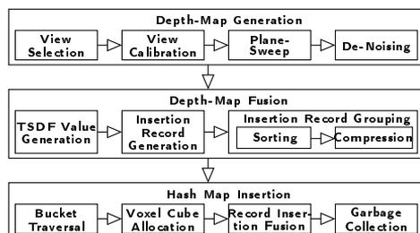
Figure 2: The three steps of the reconstruction pipeline.
