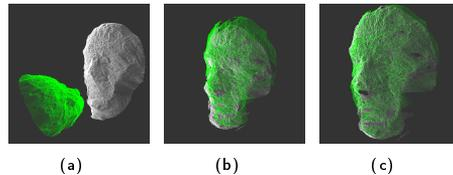
Figure 4: Registration of two example point clouds (a), after applying 4PCS (b), and after applying ICP (c).
