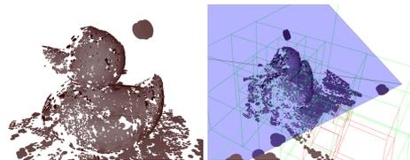
Figure 8: Left: Original camera image, right: Frustum in blue with rendered leaves in green and culled leaves in red.
