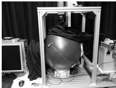
Figure 12: Hardware set-up with integrating sphere.
