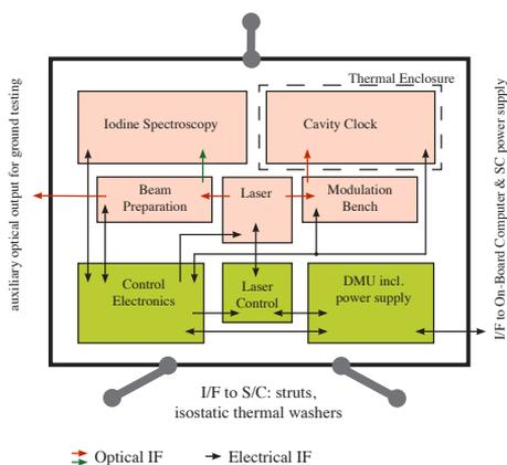
Figure 13: Functional diagram of the mSTAR payload.
