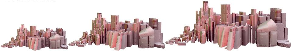
**Figure 1:** Renderings of a city voxel model stored at different level of details. The discussed data structure scheme exploits depth-map resolution and object-sensor distance for level-of-detail-aware, memory-efficient spatial data storage. This can be achieved without loss of geometric detail.
