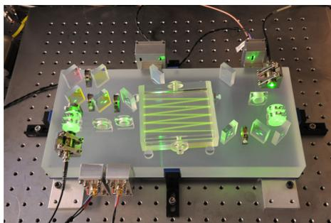
Figure 14: Photograph of the iodine spectroscopy setup.
