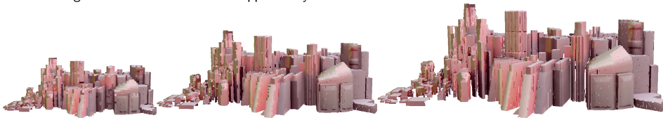
Figure 13: Renderings of a city voxel model stored at different level of details. The discussed data structure scheme exploits depth-map resolution and object-sensor distance for level-of-detail-aware, memory-efficient spatial data storage. This can be achieved without loss of geometric detail.
