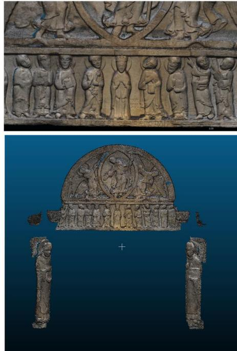
Abbildung 5: Photogrammetric reconstruction of the portal.
