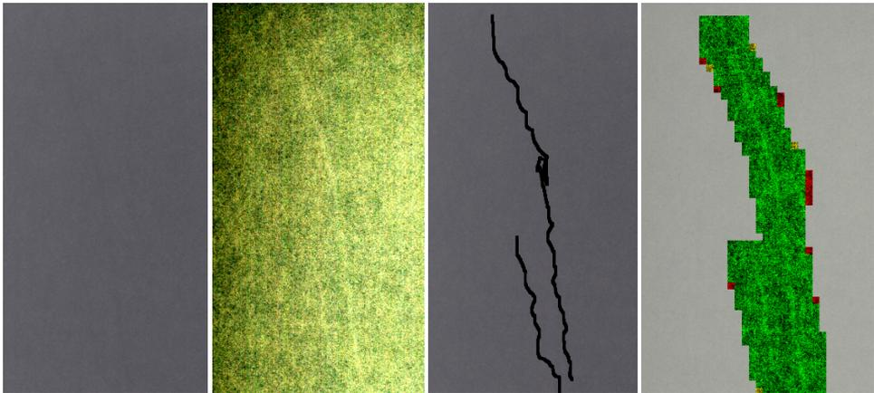
Abbildung 6: *Left*: Example of flowmarks on a laminated decor shown in the original contrast; *middle left*: Contrast maximized image of the flowmarks; *middle right*: Hand labeling for training and testing the detection system; *right*: detector output - detected regions that contain flowmarks are marked in green, erroneous detections in red.
