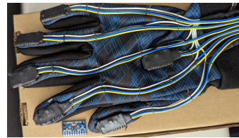
Figure 16: The glove used to demonstrate the calibration of the accelerometer data: Five IMUs are placed on the fingers, approximately at the position of the fingernails, and one IMU is located on the palm. In addition, a single IMU unit is displayed near the thumb for reference.
