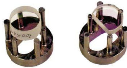
Figure 6: Measurement mirror (left) and reference mirror (right) mounted on the clamps. The reference mirror is cut in order to allow the measurement beam to pass to the measurement mirror.
