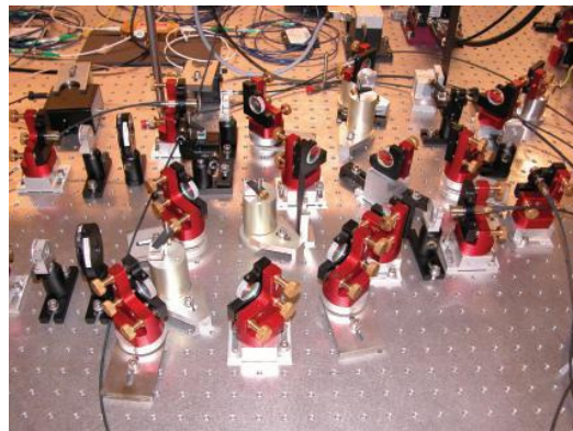
Figure 5: Photograph of the optical setup for beat measurement, Laboratory for Enabling Technologies EADS-Immenstaad.
