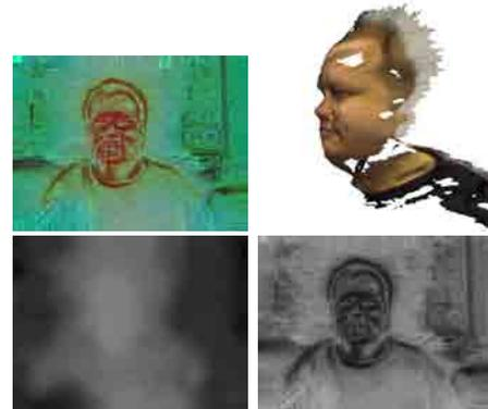
**Figure 3:** Results: All color channels (top left), reconstructed 3d model (top right), disparity map (bottom left), quality measure (bottom right).
