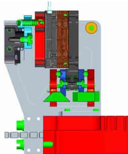
**Figure 2:** Construction of the beam actuation system
