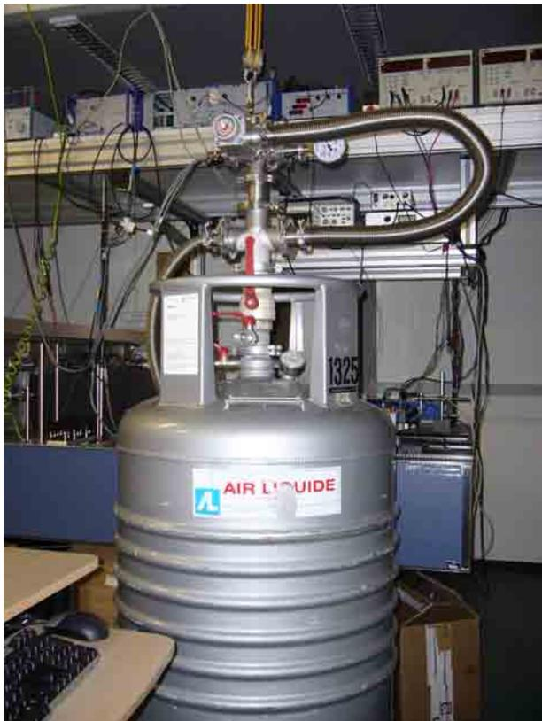
**Figure 5:** Dip stick with fibre sample on 10 K level during live test.
