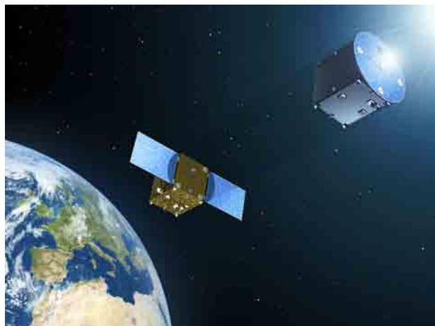
**Figure 1:** Artists view of the PROBA-3 mission. Two spacecraft in a distance of  $\sim 150$  m form a coronagraph where one spacecraft carries the occulter and the other the optical bench, electronics and detectors (figure: ESA).
