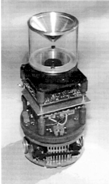
Figure 2. Khepera™ robot with camera module and custom made conical mirror, which permits sampling of the environment over  $360^\circ$ , in a range of  $\pm 10^\circ$  about the horizon.
