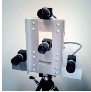
Fig. 1. The multi-camera stereo-matching system used in this paper generates one depth image from four camera images
