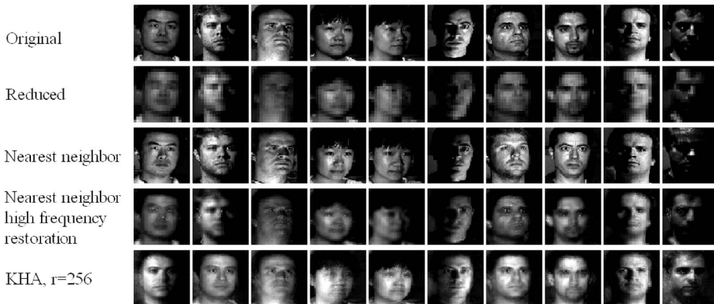
Fig. 13. Face image super-resolution based on nearest neighbor methods. First and second rows: original and low-resolution input images ( 20 \times 20 ), respectively. Third row: reconstructions obtained by replacing KPCA with a nearest neighbor classifier in the single patch reconstruction experiments. Fourth row: reconstructions obtained by the multipatch reconstruction method applied to the input image as a single patch. Fifth row: reconstructions obtained by the KHA.
