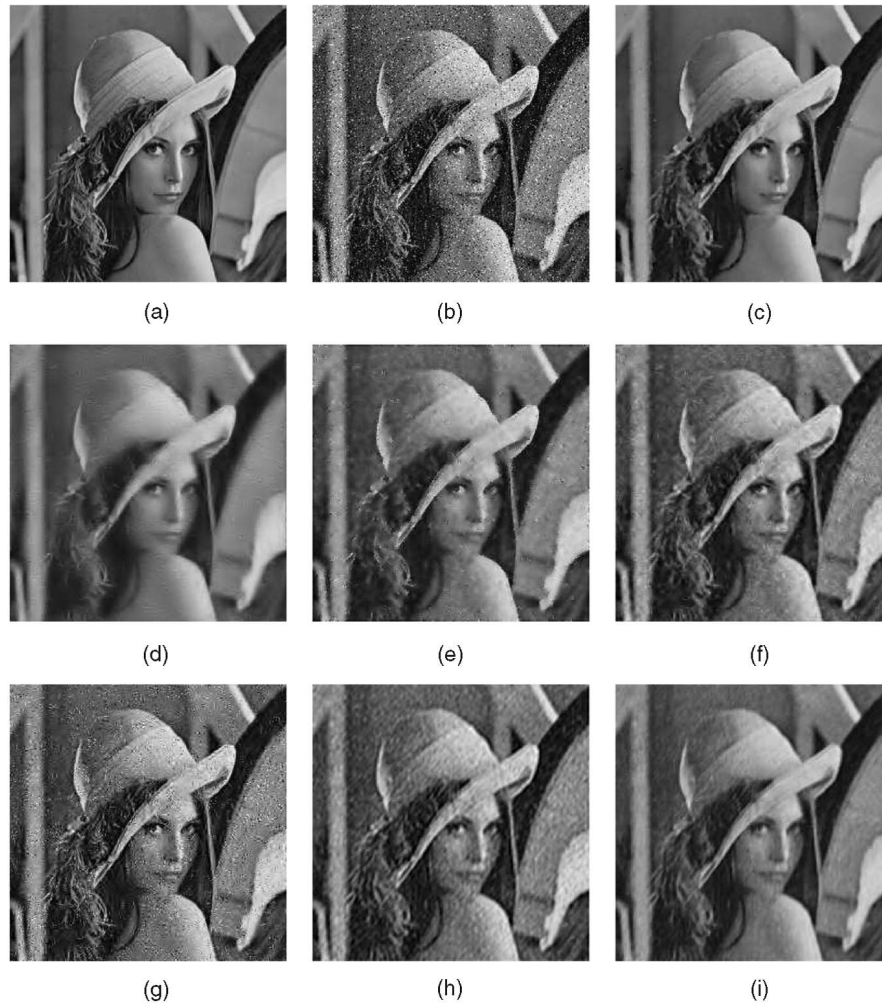
Fig. 15. Denoising salt and pepper type noise: (a) original image, (b) input noisy image, (c) median filter, (d) Matlab's wavelet denoising, (e) Matlab's Wiener filter, (f) Choi and Baraniuk's method [9] ( d = 2.0 ), (g) Pizurica and Philips's method [37] (Daubechies wavelet8), (h) PCA ( r = 20 ), and (i) KHA ( r = 20 ).
