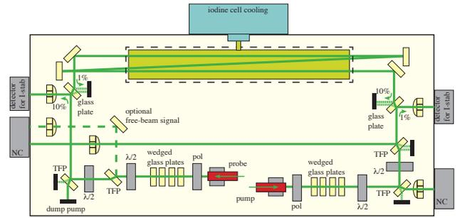
Fig. 5. Schematic of the EBB setup. The two laser beams for pump and probe are fibre-coupled to the spectroscopy board. Wedged glass plates are used for beam adjustment after integration. This setup uses a 30 cm long iodine cell in triple-pass configuration<sup>14)</sup>.
