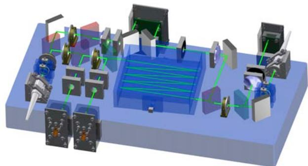
Fig. 7. 3D view of the CAD model of the EM setup. The electronics is mounted to the sides of the fused silica baseplate.
