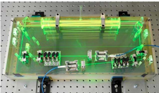
Fig. 4. Photograph of the spectroscopy unit realized on elegant breadboard level. The baseplate is made of Clearceram-HS with dimensions of 550mm x 250mm. The optical components are integrated using adhesive bonding technology<sup>14)</sup>.
