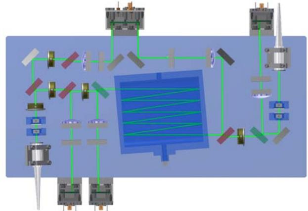
Fig. 6. Top view of the CAD model of the spectroscopy unit (engineering model level). The baseplate has dimensions of 380mm x 180mm x 40mm. The laser beam launched on the left side corresponds to the probe beam, the laser beam launched on the right side to the pump beam.
