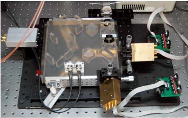
Fig. 3. Photograph of the integrated heterodyne interferometer using adhesive bonding technology. The baseplate is made of Zerodur with dimensions of 200mm x 200mm. For noise characterization, a single mirror acting as reference and measurement mirror was implemented (shown on top side of the photograph). Two quadrant photo detectors are used for tilt measurement.
