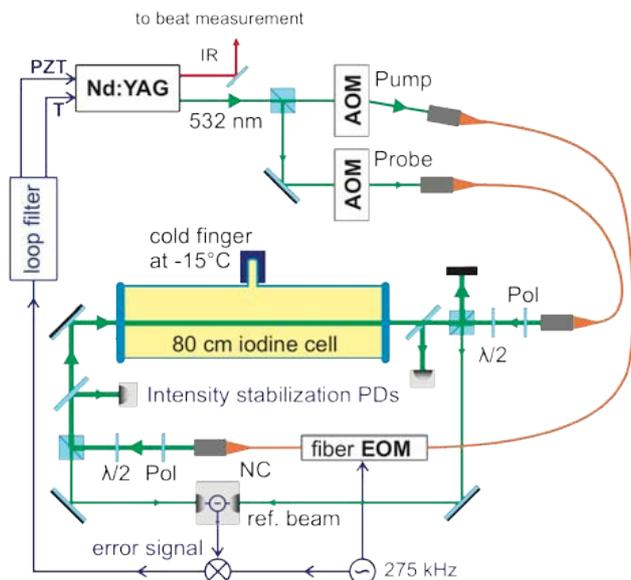
Fig. 1. Schematic of the laboratory setup of an iodine-based frequency reference using modulation transfer spectroscopy and an 80 cm long iodine cell<sup>14</sup>.
