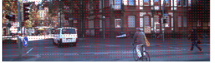
Fig. 3: Visualization of the uniform sampling grid  $\mathcal{G}$  for sub-sampling the projected Lidar points. The distance  $M_g$  between the grid points is given in pixels.
