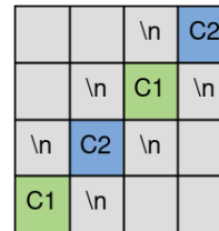
Fig. 6. Example of a text line that is incorrectly aligned along a diagonal. The correct label sequence is ‘C1 C2’ and not ‘C1 C2 C1 C2’ in this example.
